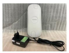
The FLUX GATEWAY communicates between the FLUX READERs and the central FLUX application. The FLUX GATEWAY is capable of buffering received data from the FLUX READERs in case the communication with the central FLUX application fails. The FLUX GATEWAY is powered on by plugging the power adapter plug into a wall socket. LED's on the side of the gateway will turn on, indicating the device is powered on.
