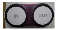
The FLUX READER is a RFID Tag Reader powered by four consumer battery (AA type). It is capable of reading Mifare cards, which info, completed with the info of the pushed button (IN / OUT) will be transmitted to the FLUX GATEWAY. This gateway is connected to the central FLUX system where all received data is processed. To use, present the RFID tag/card and press either the IN or the OUT button. A beep will sound and a green LED will blink
